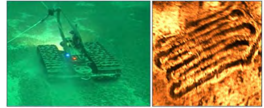
(Left) Tracked ROV deployed underwater at a 45-meter depth study location in Lake Michigan that is covered with extensive invasive mussel beds. (Right) Forward-looking multibeam image of the 100-square-meter plot cleared using the "water jet" implement pulled behind the tracked ROV. Image: NOAA
