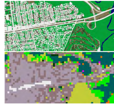
New high-resolution landcover data in places like Detroit, Michigan (top), will help resource managers make more informed restoration and protection decisions, compared to the previous regional 30-meter land cover data (bottom)
